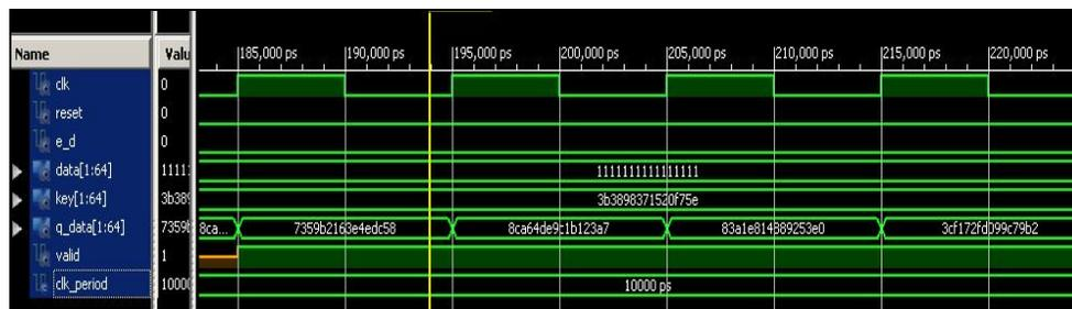
Figure 7: Waveform of DES simulation (Pipelined Mode)
