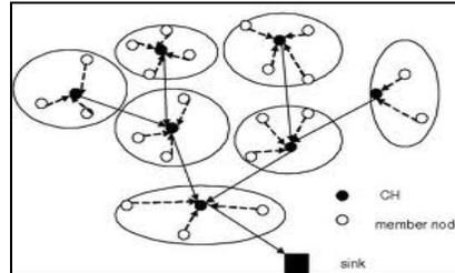
Figure 1: Data Collection using Mobile Sink through Cluster Head
