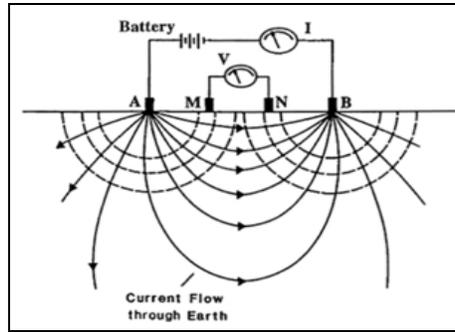
Figure 3: Typical electrode configuration for Schlumberger array.
