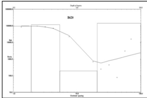
Figure 4c: Shows the VES curve at B620
