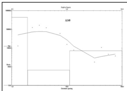
Figure 4a: Shows the VES curve at A140
