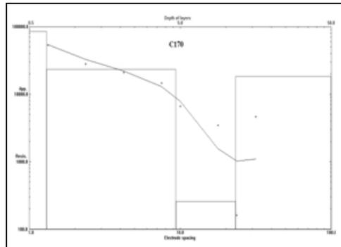
Figure 4e: Shows the VES curve at C170
