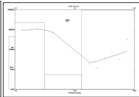
Figure 4d: Shows the VES curve at SP1
