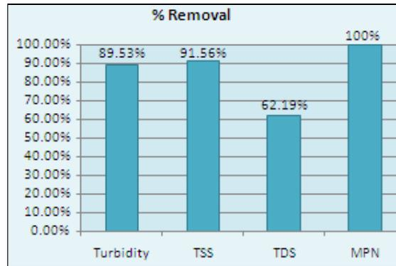
Graph 1: Removal efficiency of different parameters of different samples
