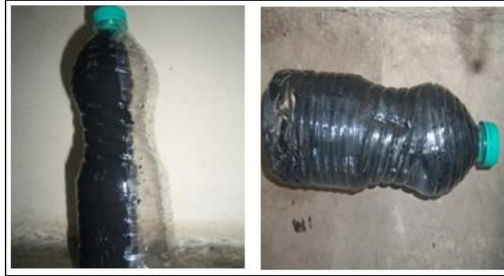
Figure 2: Half painted bottle which is used for Disinfection process
